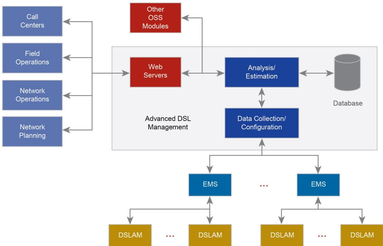
**Figure 2.** Architecture for Advanced DSL Management.
