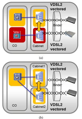
Figure 2 – An example of two DSLAMs connected via xDLV to create a larger vector group. The DSLAMs are owned by either (a) two different operators sharing the same cabinet area or (b) by the same operator.
