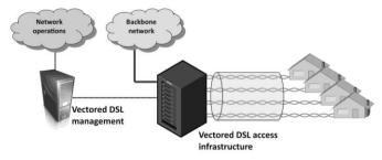
Figure 5 – Vectored DSL access infrastructure and management owned by a single provider.
