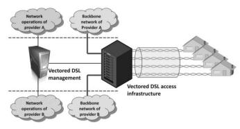
Figure 7 – Vectored DSL access infrastructure and management shared by multiple SPs. The DSLAM icon may represent a single DSLAM or also multiple ones (e.g., one or more DSLAMs per SP) and the DSLAMs of the various SPs can be cross-vectored via xDLV.
